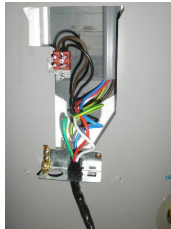
Step 3 withdraw the power cable
