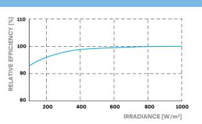
Typical panel performance under low irradiance conditions in comparison to STC conditions ( 25°C, 1000 W/m²).
